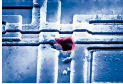
Figure 64 | Example of ESD damage
